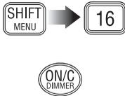
To enter security mode, press **SHIFT** followed by **16**. The display will show “NO SCRM”, if the scrambler function is not enabled in the system. If security mode is enabled, the display will show “SEC” in the top left-hand corner of the LCD.
