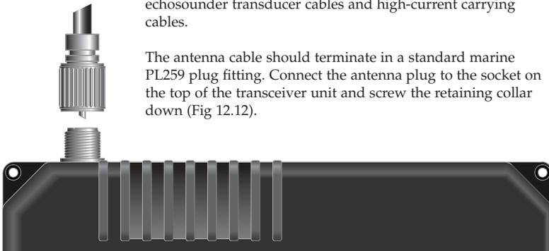
Fig 12.12 - VHF antenna connection
