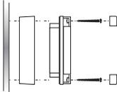
Drill a 5mm (0.2in) hole for the speaker cable. Attach the self-adhesive gasket to the back of the loudspeaker. Remove the four detachable corners which conceal the mounting holes. Fit the pattress to the back of the speaker and use the long self-tapping screws provided to fix the speaker and the pattress block to the bulkhead. Refit the corners to conceal the screw fixings.
