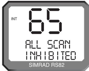
Fig 8.1 - Selected channel inhibited from scan
