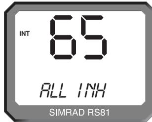
Fig 4.1 - Selected channel inhibited from scan
