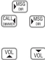
Press **▶ MSG** to access the call log menu. If the call logs are empty the display will show “NO CALLS RECEIVED” before returning to the default display. Use the **CALL ◀** and **▶ MSG** keys to switch between the standard call log (indicated by a small “1” shown next to the large digits) and the distress call log (indicated by a small “2” shown next to the large digits).
