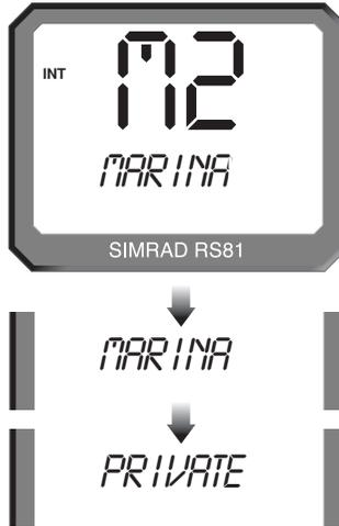
Fig 3.3 - Selecting auxiliary channel sets (sets must be available to be displayed)
