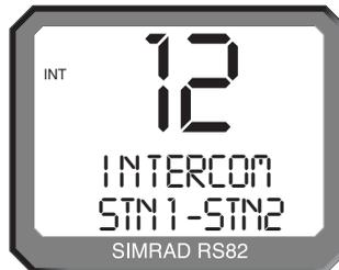
Fig 11.7 - Making an intercom call to Station 2 from Station 1
