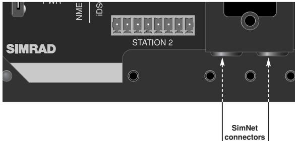
Fig 12.8 - SimNet connectors
